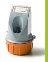
Point Orange IoT is a compact Logger/RTU device with integrated battery, a 4G modem for connections to LTE-M and NB-IoT networks, internal and/or external antenna, flexible I/O options, Modbus and SDI-12 master capability and a submersion sensor.
